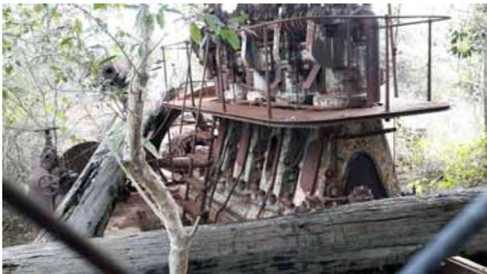
**A former ship's engine that ran an electric generator that powered an abandoned goldmine in Ravenswood FNQ.**
