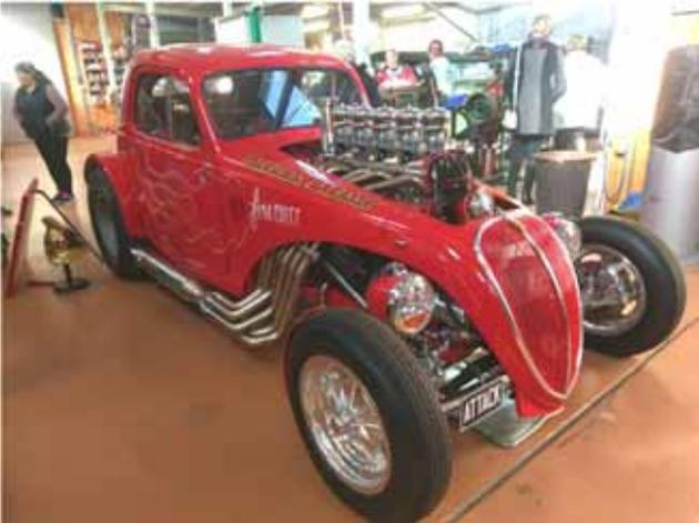
Once inside, it was amazing! A Fiat Topolino body rod with a La France fire truck side valve V12 engine, topped by five two barrel Strombergs.
