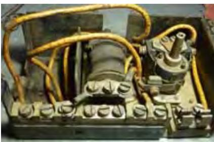
Prior to the clutch exercise I have rewired the Rotax control panel for the 'Restored Crossley' as the panel that came with the car had damaged wiring
