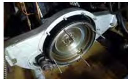
concern and will now have to wait till new clutch facings are sourced, cut to size and riveted to the driven plate. As the clutch has a large cone spring holding the pressure plate via 3 pivoted levers I have been reviewing the spare parts bin to find the best examples to refurbish while awaiting the return of the driven plates.
