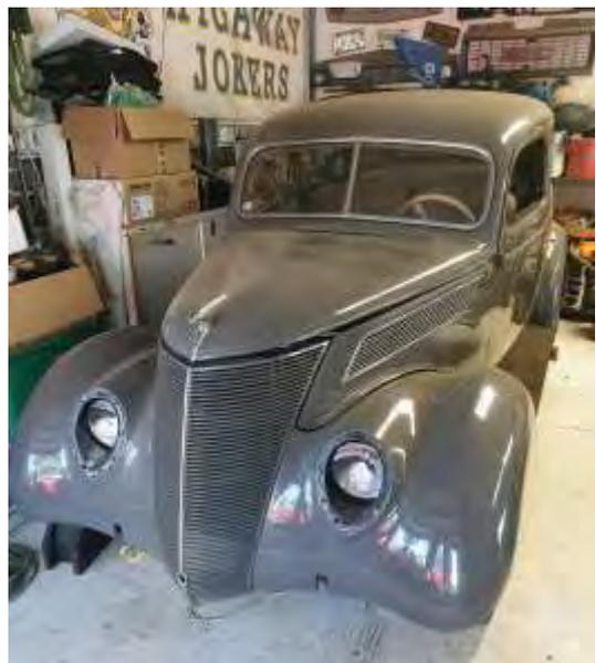
It is now in Ballarat being converted to right-hand drive. It will be restored to its original configuration, with an original flathead Ford V8, so as it can be club registered rather than a street rod registered. (Somebody had put in a 327 small block chev engine in it!) Lots of progress!
