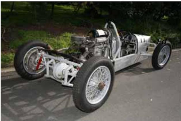
One of Hickford's other changes, which we can see in the photo, was to replace the Lancia transverse leaf spring at the rear with "coil-over-shocks" so although the engine isn't visible it must be Hickford's version of the car.
