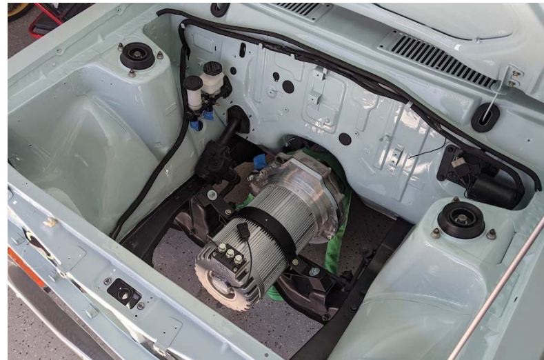
An electric motor replaces the combustion engine in the Datsun. (Supplied: Ken Macken)
