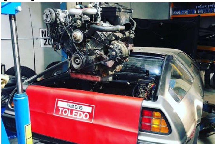
Removing the engine from the DeLorean, which is being converted to an EV. (Supplied: Electric Car Cafe)
